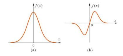
**FIGURE B.2** (a) The function  $f(x) = e^{-x^2}$  is an even function, f(x) = f(-x). (b) The function  $f(x) = xe^{-x^2}$  is an odd function, f(x) = -f(-x).
