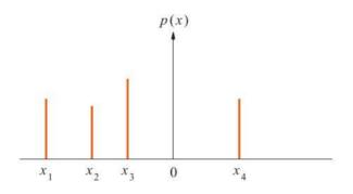
**FIGURE B.1** The discrete probability frequency function or probability density, p(x).
